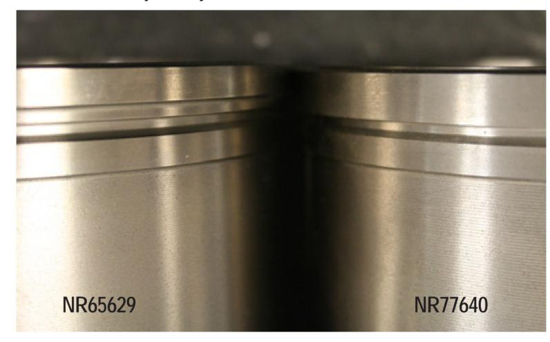
Differences in block design can be an aid in determining if your John Deere 6-619 is an early or a late model and which cylinder liners are needed for replacement.
